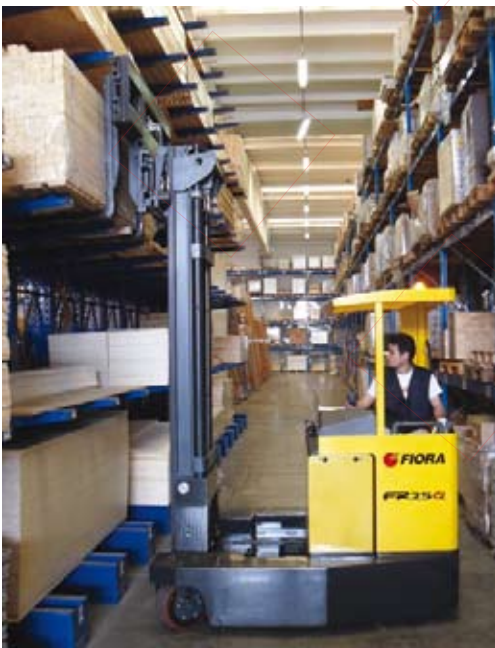
Forward / reverse travel steering all wheels after accessing aisle sideways
