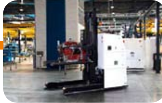
Laser-navigating 1.5t PHOENIX part of a logistic operation in motor production facility.
