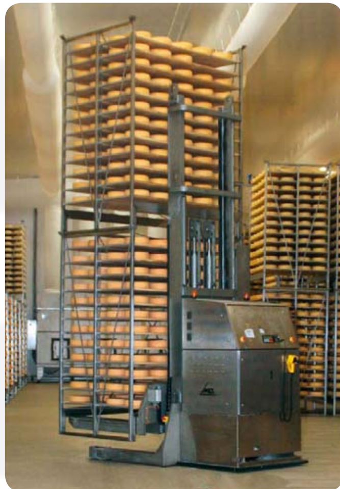
PHOENIX - stainless steel AGV with 4.6 t of cheese on the way to the ripening stage.
