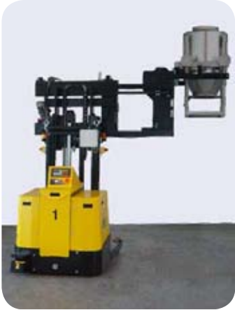
ISIS with special side shift attachment in an industrial bakery
