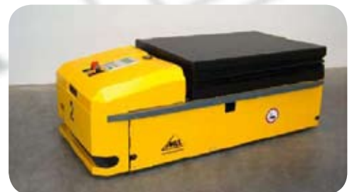
Motormouse - with electric lift platform
