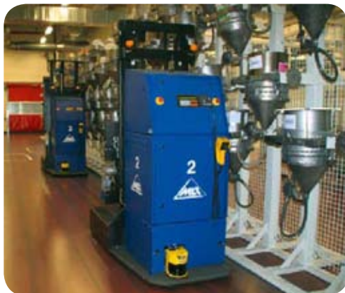
PHOENIX - delivering, transporting, metering with lift mast, scale and side shift attachment.
