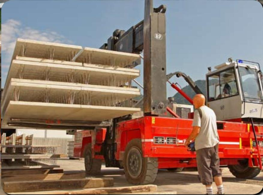
RF Remote controlled positioning shown above
